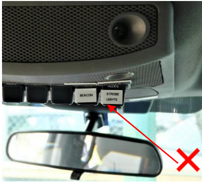
Not Acceptable – Not Permanently Label
